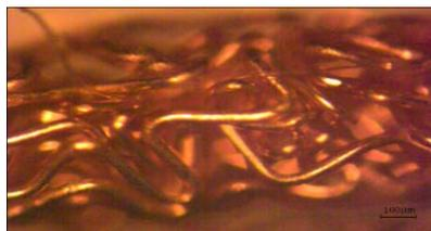
**Figure 2.** Fuzz Button connector partially enlarged.
