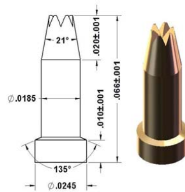
92-30712-6 Ø.0245" Base/Ø.0185" Serrated Tip
